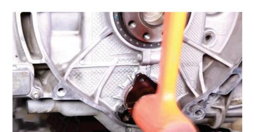
Using assembly lube, lubricate IMS Solution bearing and install IMS solution flange into bearing by hand. Then using a soft face hammer, lightly tap the IMS Solution flange until it is flush with crank case.
